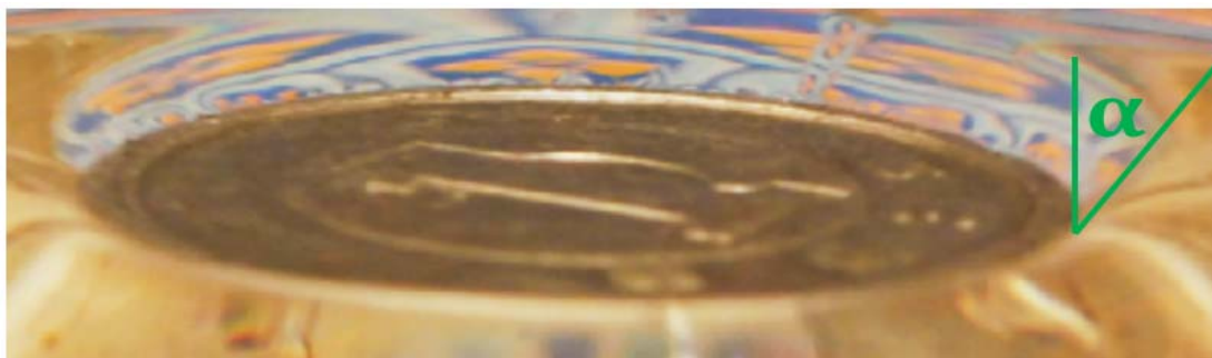
Figure 2: Macro capture detailing coin floating on the water surface. It is possible to measure the contact angle (green) and use it, together with dive ratio, to compute the combination of buoyancy and surface tension effect.
